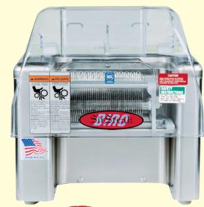
Create a value-added cube steak by moving the rear stripper (comb) to the most rear slot position. Pass 2-3 smaller pieces of hard to merchandize meat thru 2-3 times which knits the pieces together.
